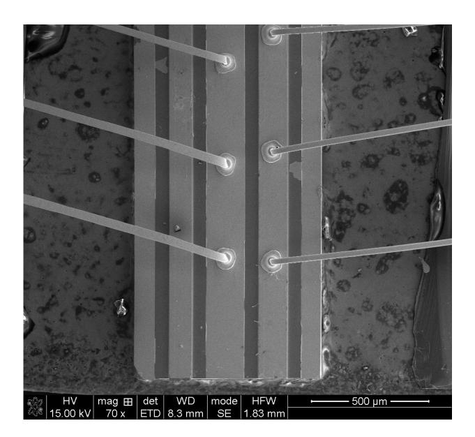
Scanning electron microscope image of the terahertz quantum cascade laser. Credit: Wang, et al/*AIP Advances*
