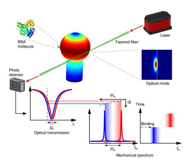
Schematic illustrating the sensing mechanism. Credit: (c) *Nature Communications* (2016). DOI: 10.1038/NCOMMS12311
