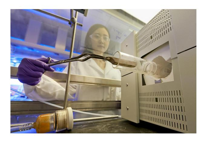
ORNL's Huiyuan Zhu places a sample of boron nitride, or "white graphene," into a furnace as part of a novel, nontoxic gas exfoliation process to separate 2-D nanomaterials. Credit: ORNL
