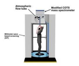
Making two measurements – vapor detection via mass spectrometer and visual image via currently deployed body scanner – in the same time and space. Credit: PNNL, CC BY
