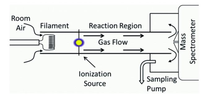
Schematic diagram of the elegant simplicity of the AFT-MS device. Credit: PNNL, CC BY
