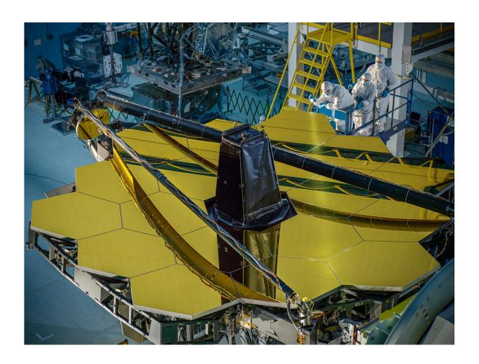
At a Goddard cleanroom, technicians unveil the James Webb Observatory's segmented mirror in preparation for an alignment test this summer. The tool used to determine the segments' alignment has inspired Goddard technologists to create another that offers picometer accuracy for next-generation observatories. Credit: NASA/Chris Gunn
