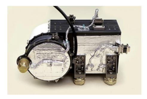
NASA's Juno spacecraft, set to arrive at Jupiter on July 4, carries three Johns Hopkins APL-built Jupiter Energetic-particle Detector Instrument, or JEDI, units. JEDI will measure charge particles accelerated to high energies within Jupiter's magnetosphere, allowing researchers to study how their interaction with Jupiter's atmosphere generates the most powerful aurora in the solar system. Credit: JHU APL
