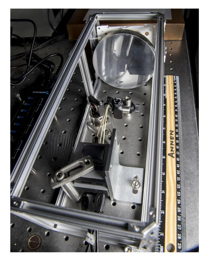
This laboratory breadboard is being used to test a conceptual telescope for use on
