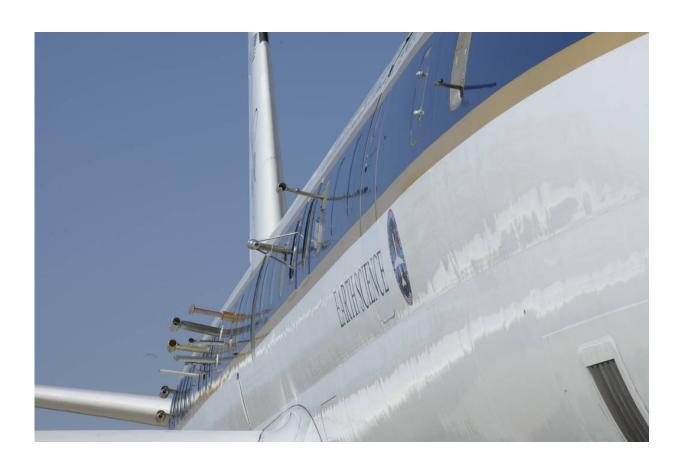
Probes on the outside of NASA's DC-8 aircraft to collect atmospheric samples. The DC-8 aircraft will be outfitted with 20 instruments for the ATom mission. Credit: NASA
