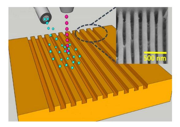
Adding aniodine or xenon difluoride gas aids nanoscale ion-beam etching of hybrid-perovskite materials. Credit: KAUST
