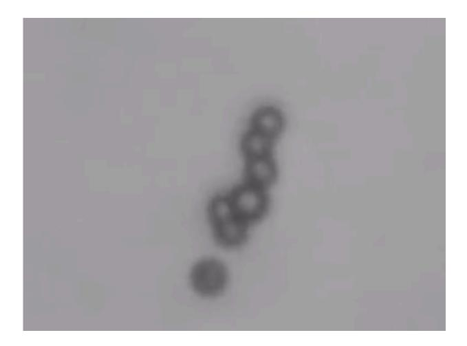
By rotating the magnetic field at a certain frequency the robotic chains will split
