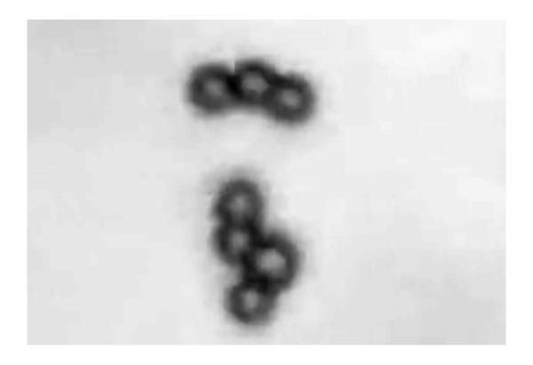
By splitting the microswimmer robot chain into separate actuated robots, multiple tasks can be completed at once. This makes them ideal for surgery and targeted drug delivery. Credit: Drexel University
