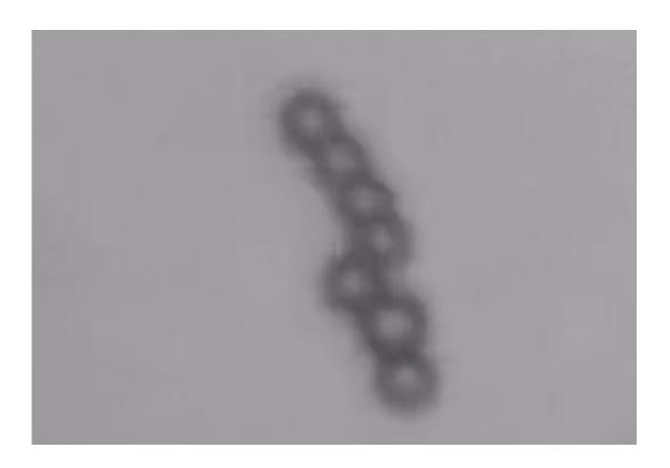
Microswimmer robots, resembling a chain of beads, can be made to move through a liquid by rotating in a magnetic field. New research shows how they can split into separate operable robots and then reconnect. Credit: Drexel University
