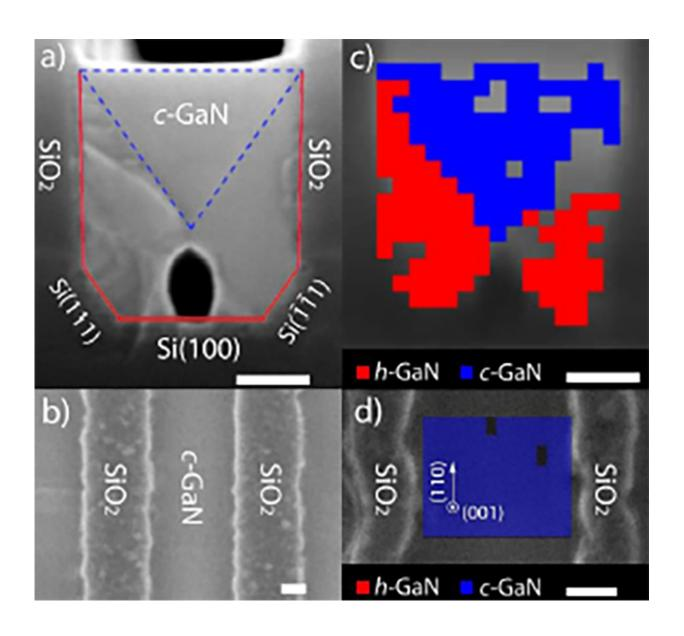
A new method of cubic phase synthesis: Hexagonal-to-cubic phase transformation. The scale bars represent 100 nm in all images. (a) Cross
