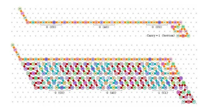
Oritatami binary counter: It cotranscriptionally folds a periodic sequence 0-1-2-... - 59-0-1-2-... of 60 abstract molecule (bead) types. (Top) The initial count 000 is encoded as a sequence of four bead types. (Bottom) One zig-zag amounts to increment by 1, exposing different bead types below, encoding 001. After one more zig-zag, other bead types encoding 010 would be exposed below, and so on. Credit: University of Electro-communications
