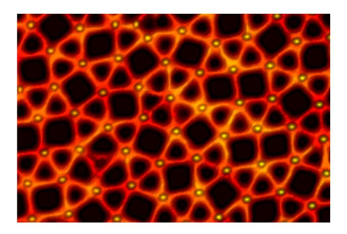
Scanning tunneling microscopic image of the quasicrystalline network built up with europium atoms linked with para-quaterphenyl-dicarbonitrile. Credit: J. I. Urgel / TUM
