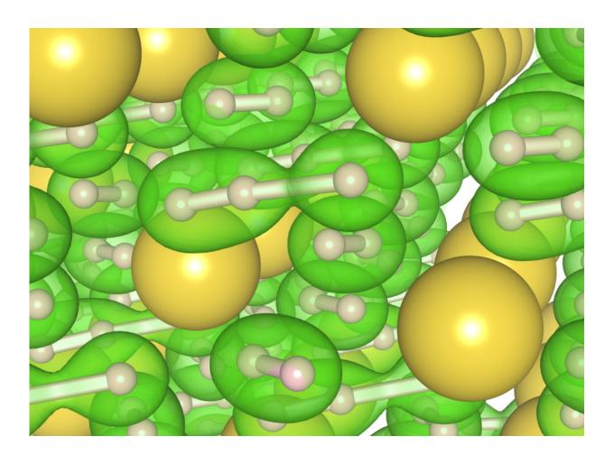
At center, in green, is the new three-atom hydrogen 'chain.' It is surrounded by several 'normal' two-atom molecules of hydrogen, also in green. The new chain configuration appears in the new material NaH7, which was produced under high pressure and high temperature conditions. The new material could change the superconductivity landscape and be useful for hydrogen storage in hydrogen fuel cells. Credit: Duck Young Kim
