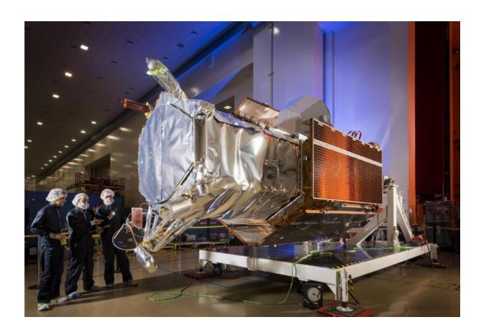
Built by Lockheed Martin, the WorldView-4 satellite will expand DigitalGlobe's industry-leading constellation of high-accuracy, high-resolution satellites, and double the availability of 30 cm resolution imagery for commercial and government customers around the globe. Credit: Lockheed Martin
