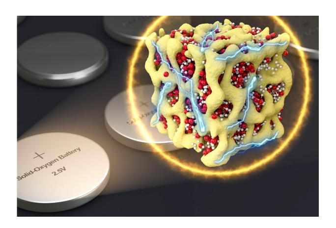
In a new concept for battery cathodes, nanometer-scale particles made of lithium and oxygen compounds (depicted in red and white) are embedded in a sponge-like lattice (yellow) of cobalt oxide, which keeps them stable. The researchers propose that the material could be packaged in batteries that are very similar to conventional sealed batteries yet provide much more energy for their weight. Credit: Courtesy of the researchers
