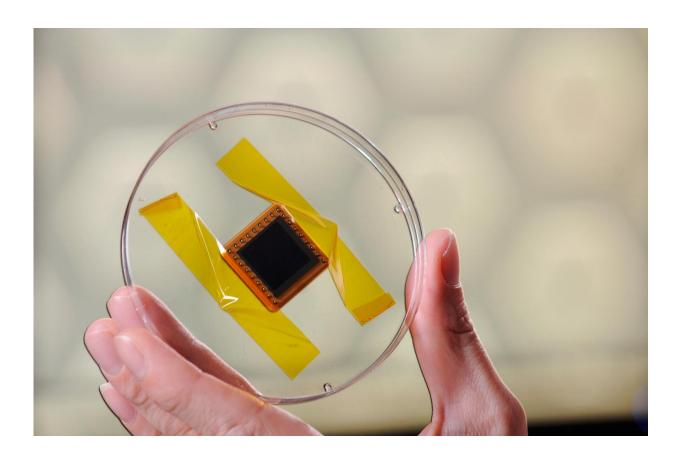
Photo shows a solar cell produced for space testing of new types of photovoltaic cell materials aboard the International Space Station. Credit: Gary Meek, Georgia Tech
