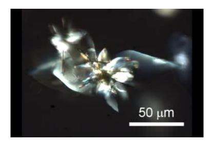
Microscopy of self-oscillation of the crystalline assembly. A crystalline assembly of azobenzene derivative and oleate showed oscillatory bending-unbending motion under continuous 435-nm light irradiation. The frequency of oscillation increased with increasing light intensity. Credit: Ikegami T. et. al., Angewandte Chemie International Edition, May 19, 2016
