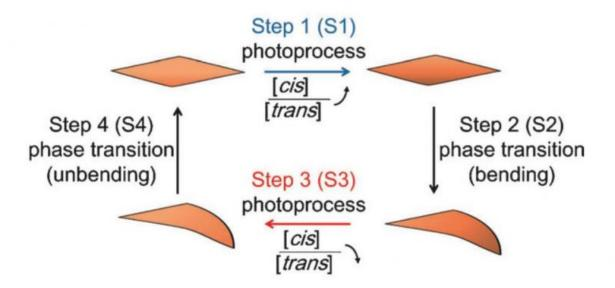
Schematic illustration of each step of the self-oscillatory motion. Credit: Ikegami
