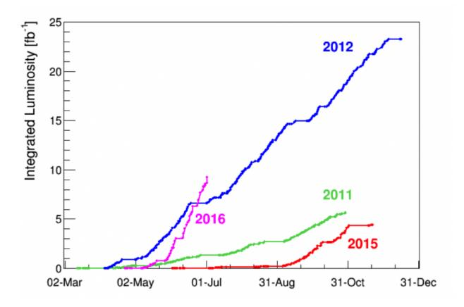
This graph shows the integrated luminosity delivered by the LHC to the ATLAS and CMS experiments in 2011, 2012, 2015 and 2016. The integrated luminosity indicates the amount of data delivered to the experiments and is measured in inverse femtobarns. One inverse femtobarn corresponds to around 80 million million collisions. Credit: CERN
