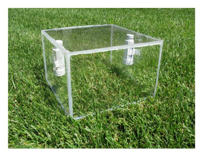
Litvak's mini-chamber was used to measure ET in urban lawns. Credit: Elizaveta Litvak
