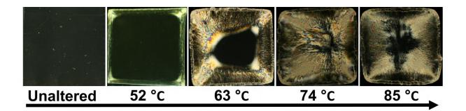
Treating polylactic acid, a commonly used polymer material, with heat and pressure creates crystals and causes polymer strands to become more organized. Those changes could make the material more useful in medical applications. Credit: Mathiowitz lab / Brown University
