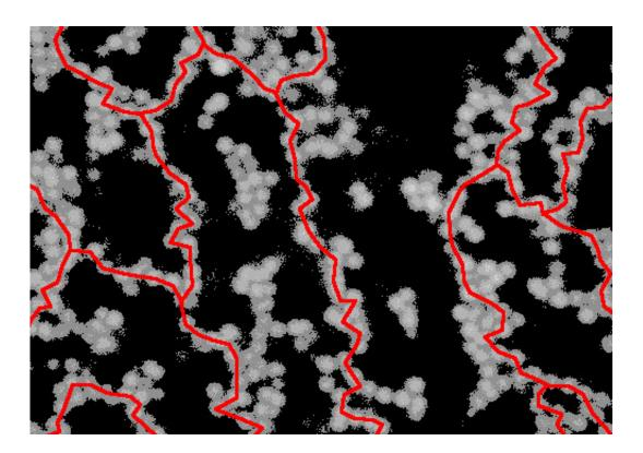
An image of a colloidal gel taken with a confocal microscope. Directed chains of particles (shown in red) that span the whole system are required for gels like this to form. Credit: Ronja Capellmann/Michael Schmiedeberg
