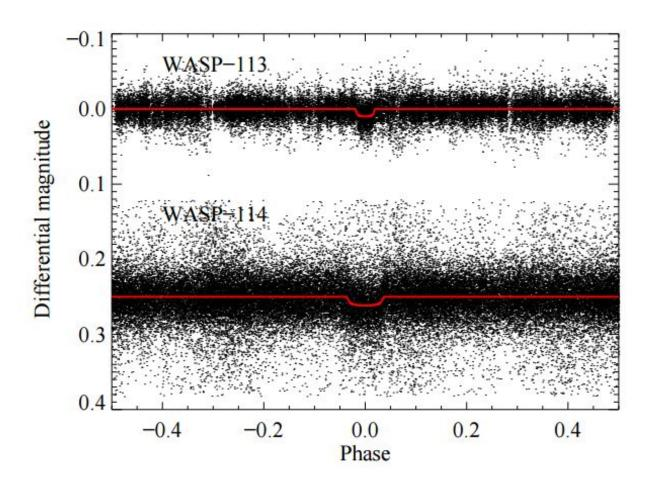
SuperWASP phase folded light curve for WASP-113 (top) and WASP-114 (bottom). The best transit model described in detail in section 4 is overplotted. The data of WASP-114 was displaced vertically for clarity. Credit: arXiv:1607.02341 [astro-ph.EP]
