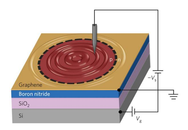
The STM tip spatially probes Dirac fermion wavefunctions in the presence of the p–n junction. Credit: (c) *Nature Physics* (2016). DOI: 10.1038/nphys3805
