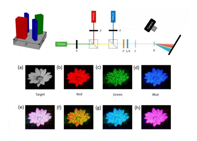
(Top left) One pixel, which is made of four nanoblocks. (Top right) Experimental setup for generating a color hologram. (Bottom) Experimental results of achromatic color holograms, made of red, green, or blue light or by combining these colors. Credit: Wang et al. ©2016 American Chemical Society
