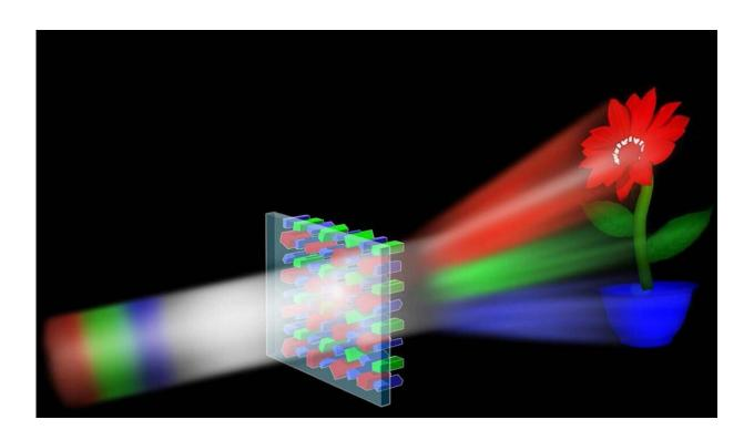
Color holographic image made by shining laser light on a metasurface. Credit: Wang et al. ©2016 American Chemical Society
