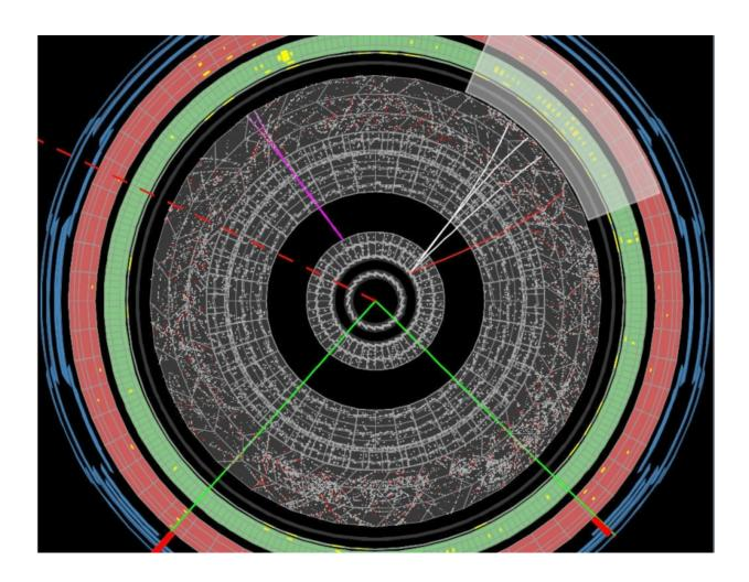
These images show how particles appear in the ATLAS detector. The lines show the paths of charged particles travelling away from a collision at the centre. Volunteers are looking for tracks appearing 'out of thin air' away from the centre. Credit: CERN
