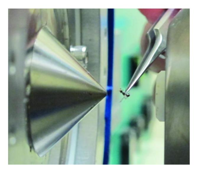
Analysis of a single fly using mass spectrometry. The fly is held by forceps in the mass spectrometer inlet. This form of analysis revealed that knockdown of spidey resulted in a near-complete loss of hydrophobic waxes on the insect surface. Credit: Chiang, et al. (2016)
