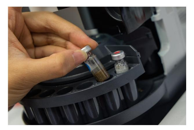
Prepared soil samples used to test bioengineered tools that will allow researchers to study Earth's microbes from micro- to macroscales. Rice University researchers have developed microbial sensors that release gas to report on specific biochemical reactions. Credit: Jeff Fitlow/Rice University
