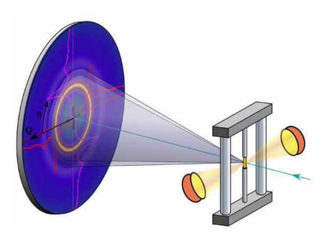
Typical 2D high-energy x-ray diffraction setup: a small beam arriving from the right is scattered by the specimen into Debye–Scherrer cones, which are mapped as diffraction rings on a flat-panel detector. Superimposed to the 2D detector image are four radial sections of the intensity. The specimen is in a mechanical load frame, heated by halogen lamps; however, a vast variety of sample
