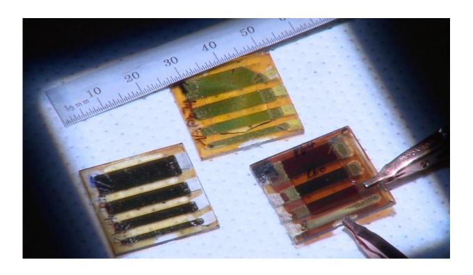
Three types of large-area solar cells are made out of two-dimensional perovskites. At left, a room-temperature cast film; upper middle is a sample with the problematic band gap, and at right is the hot-cast sample with the best energy performance. Credit: Los Alamos National Laboratory
