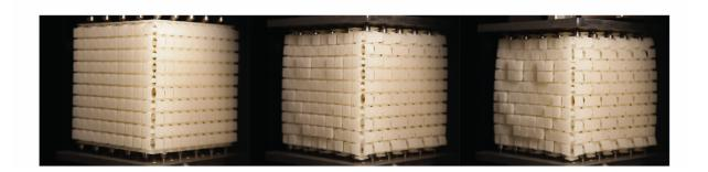
To demonstrate that any pattern can be produced on a cube's surface, the researchers developed a cube of 10x10x10 blocks on which a smiley appears when the cube is compressed. Credit: Corentin Coulais
