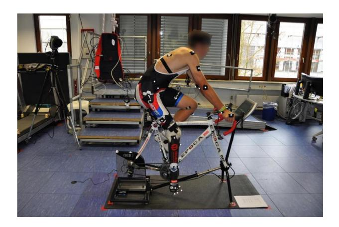
A cycloergometer and a test prosthesis help optimize prosthetics for athletes. Credit: Fraunhofer IPA
