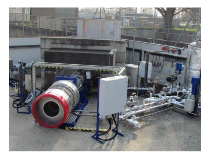
Testing the precooler design for the SABRE engine, undertaken at Reaction Engines' site in Oxfordshire in November 2012 and overseen by ESA. Credit: Reaction Engines Ltd
