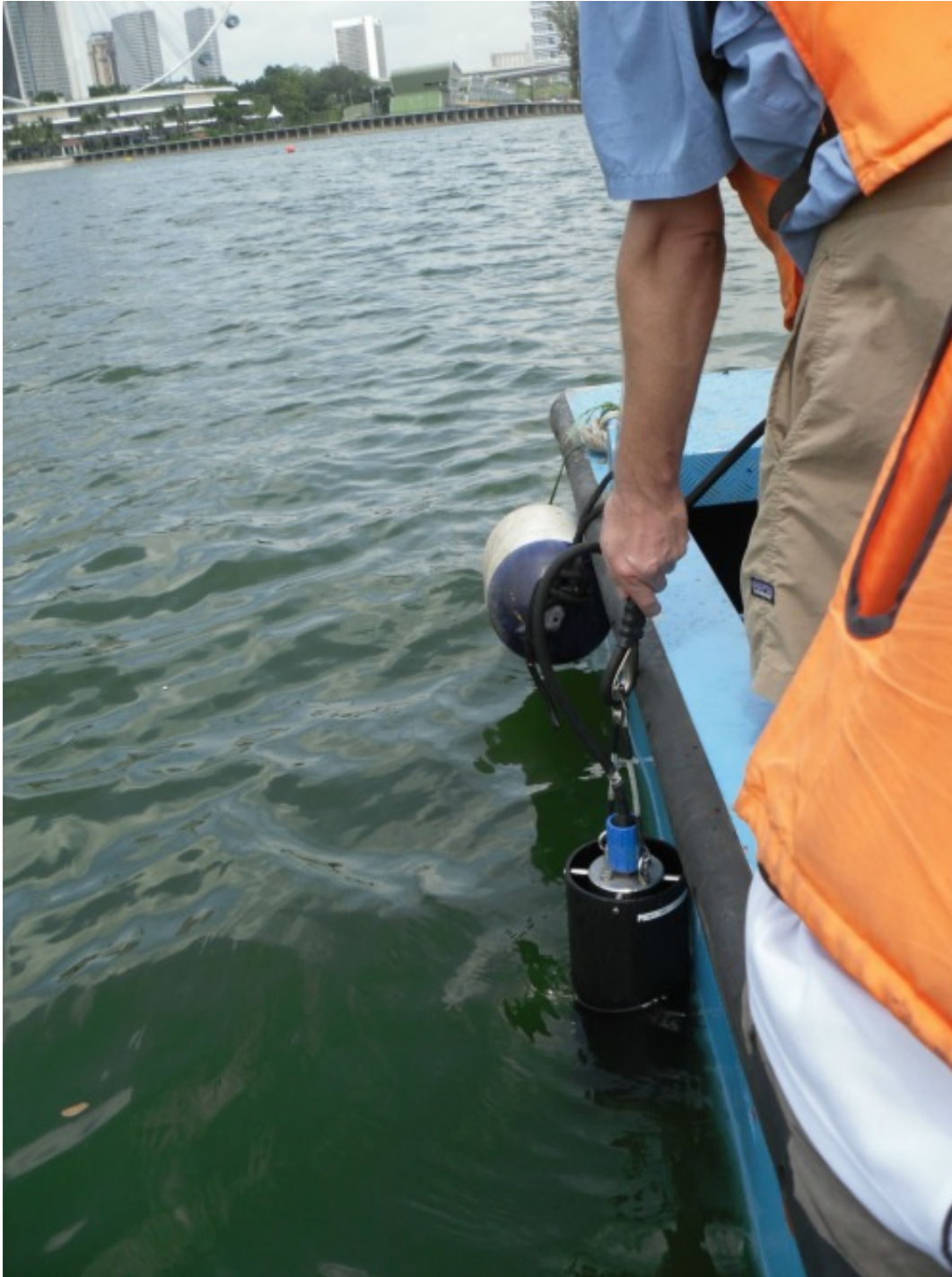
Environmental consultants Dr Hans Eikaas and Dr Jason Antenucci on the Marina Bay Reservoir in Singapore, right in the downtown area launching a gallium nitrate phytoplankton sensor for measuring algal types. Credit: DHI Water & Environment
