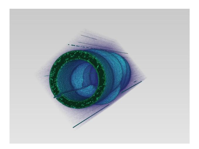
A three-dimensional depiction of the spatial variation of the optical electromagnetic field around a microantenna following excitation with terahertz pulse. The optical field is mapped with the aid of electron pulses. Credit: Dr. Peter Baum
