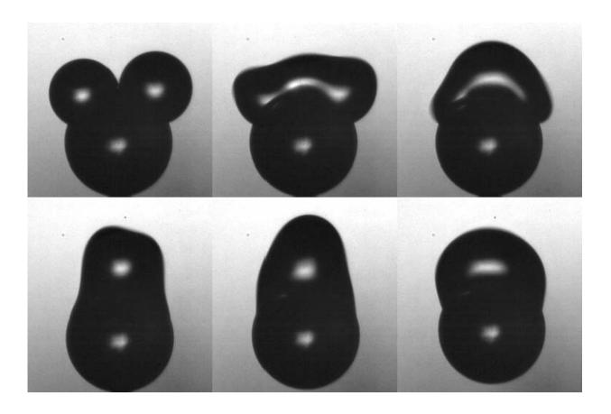
Coalescence of two water drops on a polystyrene particle leads to the launching of the particle away from the supporting substrate. Credit: Roger L. Chavez/Duke University
