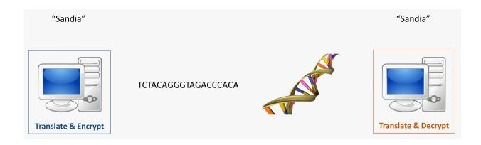
The Bachands' method of encrypting a message into DNA. Using a computer algorithm they can encrypt a message into a sequence of DNA. Then they chemically synthesize the DNA. The DNA can be read by DNA sequencing, and then translated and decoded using the same computer algorithm. Credit: Sandia National Laboratories
