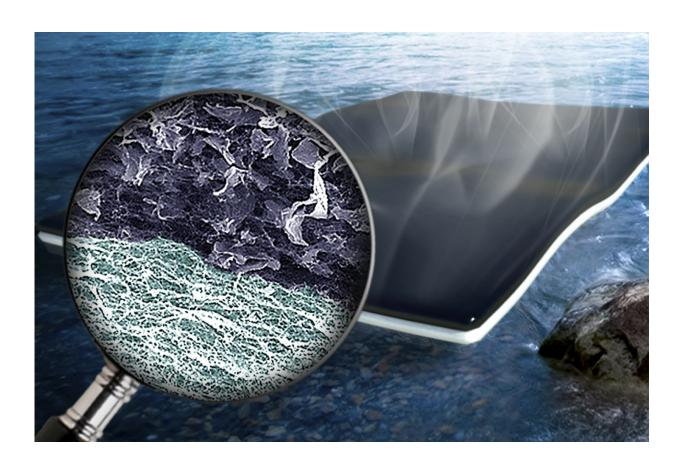
An artist's rendering of nanoparticle biofoam developed by engineers at Washington University in St. Louis. The biofoam makes it possible to clean water quickly and efficiently using nanocellulose and graphene oxide. Credit: Washington University in St. Louis
