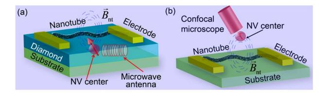
Two proposed set-ups for an experiment in which the nitrogen-vacancy (NV) center in a diamond nanocrystal is coupled to a nanotube with an electric current flowing through it: (a) the nanotube is suspended above the diamond, and (b) the diamond is above the nanotube. Credit: Li et al. ©2016 American Physical Society
