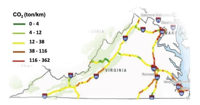
Roughness- and deflection-induced excess carbon dioxide emissions on Virginia's Interstate Highway network in 2013. Credit: Massachusetts Institute of Technology
