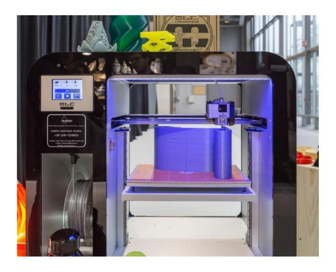
A 3D Printing device layers polymers to build an object by depositing material in very small layers. A new paper by a team of NYU Tandon researchers reports that 3D printing is vulnerable to the insertion of fine defects. Credit: New York University
