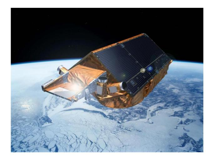
The CryoSat mission provides data to determine the precise rate of change in the thickness of the polar ice sheets and floating sea ice. It is capable of detecting changes as little as 1 cm per year. The information from CryoSat is leading to a better understanding of how the volume of ice on Earth is changing and, in turn, a better appreciation of how ice and climate are linked. Credit: ESA – P. Carril
