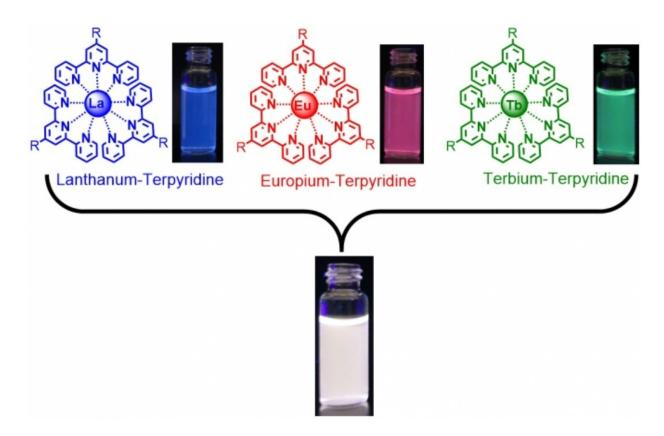
Figure 1: These samples show the effect of mixing different lanthanide ions with a ligand material called terpyridine in a solvent. In the top three vials, the lanthanides used are (left to right) lanthanum, europium, and terbium. The fluids display the characteristic colors of those elements. The white-light-emitting fluid in the lower vial was formed by mixing together equal volumes of the blue, red, and green samples above. Credit: Massachusetts Institute of Technology
