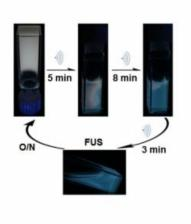
Figure 2: As one test of stimulus response, the researchers immerse samples of their white-light-emitting gel in an ultrasonic bath. Within a few minutes, the samples begin to change from gels to fluids as the complexes holding the polymer together break down. As shown, the remaining gel emits white light, while the fluid shines blue — the color emitted by the now-unbound ligands. At 16 minutes, the sample is entirely blue liquid. Left overnight, the complexes
