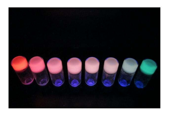
Fluorescent gels could be used as sensors for detecting structural failure in energy-related equipment. These gels were synthesized by mixing a polymer (polyethylene glycol) and a ligand (terpyridine) with two lanthanides — europium and terbium — in varying ratios. The red sample at the far left contains only europium, while the blue-green sample at the far right contains only terbium. A white-light-emitting gel forms when the mixing ratio of terbium
