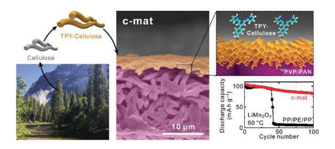
Cellulose that originates from plant material is used as a thin layer in a new separator membrane for batteries, resulting in a large increase in capacity retention at high temperatures. Credit: Kim et al. ©2016 American Chemical Society
