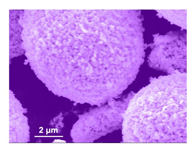
SEM image of lithium-rich cathode particles treated with a carbon dioxide-based gas mixture to introduce oxygen vacancies on the surface. Credit: Laboratory for Energy Storage and Conversion, UC San Diego
