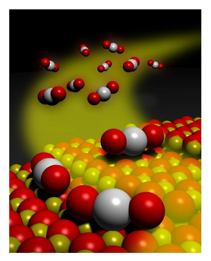
Mobile platinum oxide species trapped on a cerium oxide surface. The bonding of the platinum to surface oxygens creates isolated platinum atoms that are
