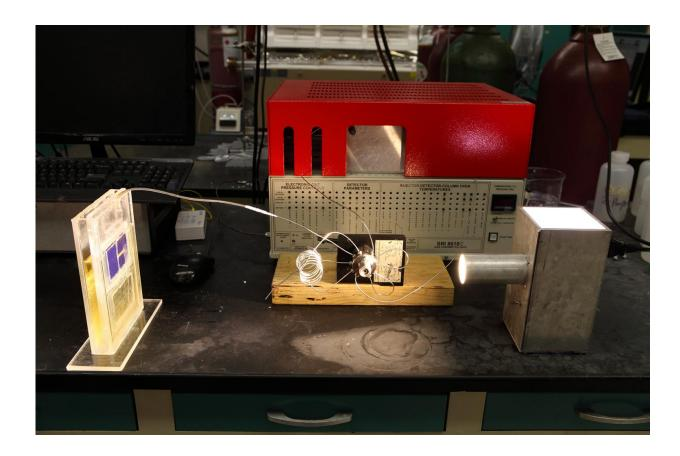
Simulated sunlight powers a solar cell that converts atmospheric carbon dioxide directly into syngas. Credit: University of Illinois at Chicago/Jenny Fontaine
