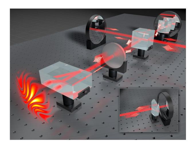
Scheme of the experimental setup for measuring holograms of single photons at the Faculty of Physics, University of Warsaw. (The experiment started with a pair of photons with flat wavefronts and perpendicular polarizations. The different polarization made it possible to separate the photons in a crystal and make one of them 'unknown' by curving their wavefronts using a cylindrical lens. Once the photons were reflected by mirrors, both photons were directed towards
