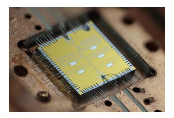
The multi-qubit chip has five superconducting transmon qubits and associated readout resonators. When cooled to absolute zero, such a device can compute things like quantum simulations of advanced materials. Credit: Quantum Nanoelectronics Laboratory, Lawrence Berkeley National Laboratory
