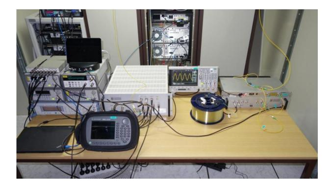
UWA's prototype SKA frequency synchronisation system alongside ancillary equipment deployed in the Compact Array's correlator room. Credit: Sascha Schediwy
